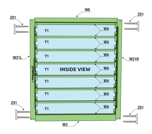
**NOTE:** Louver may be installed during construction or on a fully assembled Grandio Greenhouse. If installing during construction, it is recommended to place the louver while installing the panels in your desired location. If installing after construction, you will need to cut the panel of choice out of the greenhouse. A utility blade or jigsaw is recommended.
