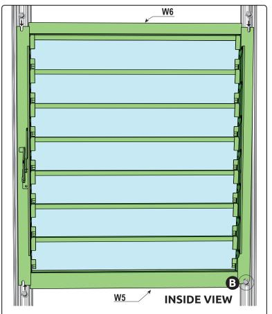
**Note:** Polycarbonate panel will sit inside the **W5** or **W6** extrusion one end may fit snug to the greenhouse extrusion, or both top and bottom may have panels. It will depend on placement how you will cut your panels.
