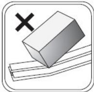
Handle with care! Dropping can bend the frame, and it will not fit properly.
